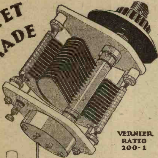
Fixed vanes insulated from end plates by porcelain.
