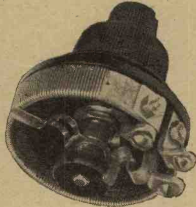
Showing the construction of the combined filament rheostat and L.T. switch received from King Quality Products, Inc.
