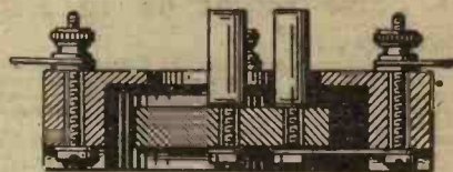
In this Etherplus valve holder the sockets are mounted on a rubber base.
